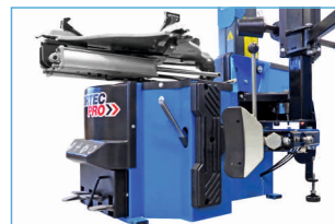
Strong bead breaker with a force of 3 tons
