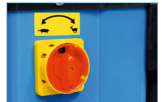
Double speed rotary table, controlled in a switch
