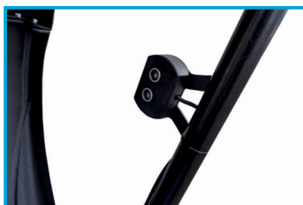
SONAR TO MEASURE THE RIM WIDTH
