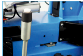
Push-button controlled bead breaker
