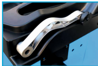
ARM FOR AUTOMATIC MEASURING THE DISTANCE AND THE DIAMETER OF THE WHEEL
