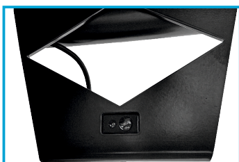
LASER TO MEASURE THE RIM WIDTH
